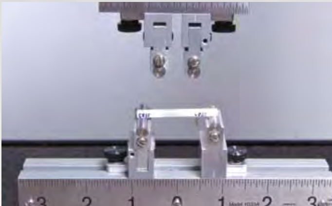
This Instron machine provides the measurement of a material's mechanical properties, including flexural, fracture and tensile strength.
